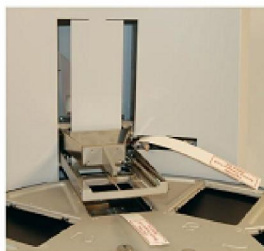
Figure 31 Both transport locks refitted
